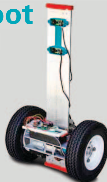
Sedgeway-like robot provides 3D map and temperature data to assist first responders
